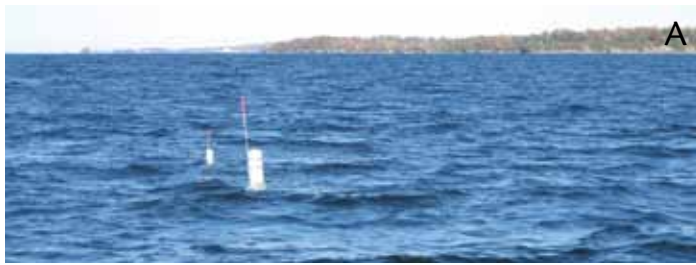
Figure 3. (A) Drogues and drifters are often deployed in pairs to show their net divergence over time as well as to provide optimal post processing for the drifter data. (B) Downloading data from the 10 GPS units can take up to half an hour, so this process must start immediately upon recovery.
